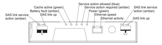
Figure 36. Controller LEDs
